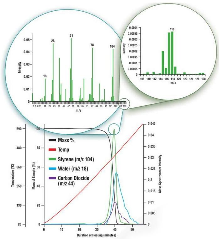
Figure 3. The thermal decomposition of polystyrene
