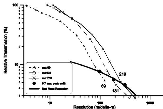
Figure 3 Relative transmission curves for 9.5 mm quadrupole (grounded entrance lens).
