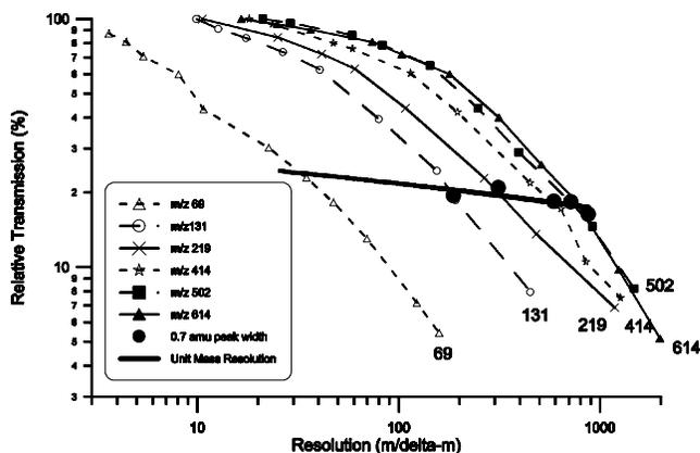
Figure 4 Relative transmission curves for 9.5 mm quadrupole (mass programmed entrance lens).
