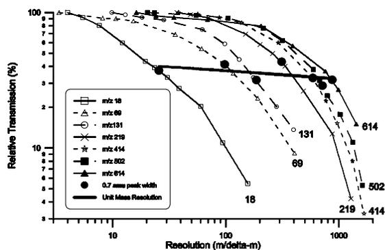
Figure 5 Relative transmission curves for 9.5 mm tri-filter quadrupole (with pre- and post- filters).
