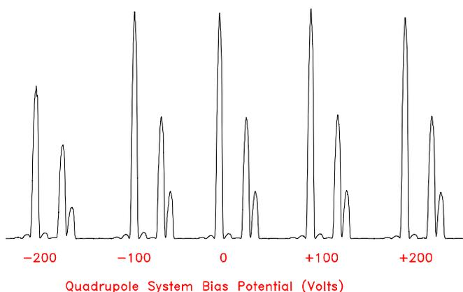
**Figure 5.** Quadrupole peak shapes with biased quadrupole housing and control electronics.
