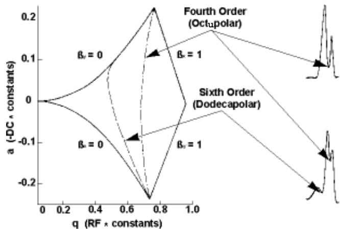
**Figure 4.** Mathieu stability diagram showing characteristic octupolar and dodecapolar non-linear resonance lines. These non-linear resonance lines correlate well with experimental peak shapes shown. Adapted from Reference 2.
