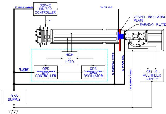
**Figure 1.** Schematic of Extrel Quadrupole probe assembly with electrically isolated quadrupole housing and electrically biased control electronics. Modifications from standard design include the addition of a vespel insulating plate between the multiplier housing and quadrupole housing, and a modified exit lens design.
