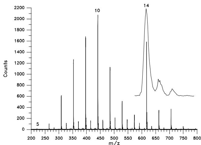
**Figure 7.** Typical  $\text{CO}_2$  anion cluster spectrum from Johns Hopkins system. Quadrupole mass analyzer and control electronics were isolated -390 Volts from ground. Labels indicate number of  $\text{CO}_2$  atoms in cluster. Inset illustrates excellent peak shape for  $(\text{CO}_2)_{14}$ .
