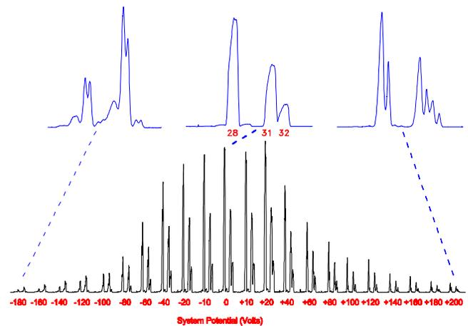
**Figure 2.** Quadrupole peak shapes with grounded quadrupole housing and biased control electronics.
