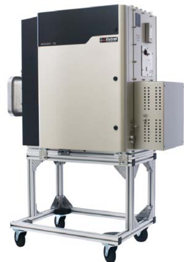
Figure 1. The MAX300-AIR is an environmental mass spectrometer capable of performing quantitative analysis on a wide variety of compounds at concentrations ranging from 10 ppt* to 100%. The system is optimized for fully-automated, continuous analysis in hazardous industrial settings.
