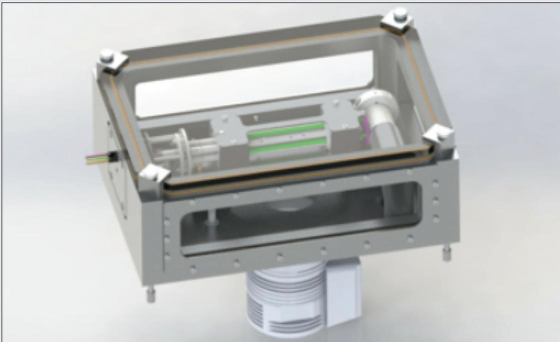
Figure 8.1.1: The capillary inlet configuration for the IQ-2000 vacuum chamber and internal components.
