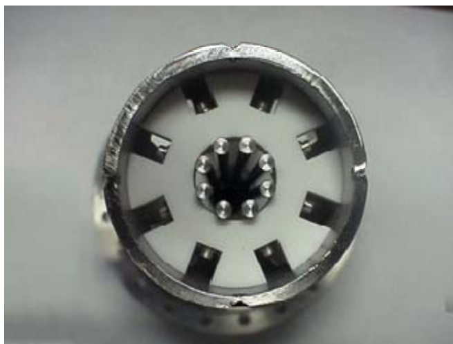
Figure 2. End view of 3 mm diameter rod octupole mass filter. Inscribed radius is 4.5 mm.
